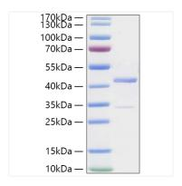
Recombinant Human PCBP1 Protein was determined by SDS-PAGE with Coomassie Blue, showing a band at 40-50 kDa.
