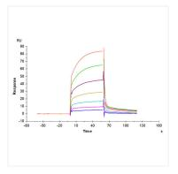
Cynomolgus PD-1, hFc Tag captured on CM5 Chip via Protein A can bind Cynomolgus PD-1, His Tag with an affinity constant of 1.28  $\mu$ M as determined in SPR assay (Biacore T200).
