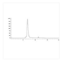
The purity of Recombinant Mouse IFN-gamma Protein is greater than 90% as determined by SEC-HPLC.
