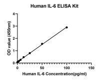
This standard curve is only for demonstration purposes. A standard curve should be generated for each assay.
