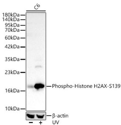
Western blot analysis of lysates from C6 cells using Phospho-Histone H2AX-S139 Rabbit pAb (AP0099) at 1:400 dilution. C6 cells were treated with UV at room temperature for 15-30 minutes. Secondary antibody: HRP-conjugated Goat anti-Rabbit IgG (H+L) (AS014) at 1:10000 dilution. Lysates/proteins: 25 µg per lane. Blocking buffer: 3% nonfat dry milk in TBST. Detection: ECL Basic Kit (RM00020). Exposure time: 20s.
