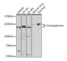
Western blot analysis of various lysates using Ceruloplasmin Rabbit pAb (A7658) at 1:1000 dilution. Secondary antibody: HRP-conjugated Goat anti-Rabbit lgG (H+L) (AS014) at 1:10000 dilution. Lysates/proteins:  $25\mu g$  per lane.
