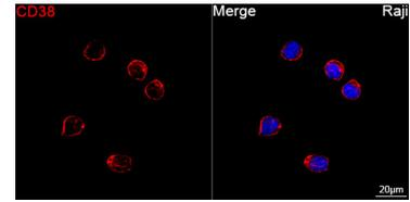
Confocal imaging of Raji cells using CD38 Rabbit mAb (A25398, dilution 1:200) followed by a further incubation with Cy3-conjugated Goat anti-Rabbit IgG (H+L) (AS007, dilution 1:500) (Red). DAPI was used for nuclear staining (Blue). Objective: 100x.
