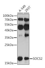
Western blot analysis of various lysates using SOCS2 Rabbit pAb (A17035) at 1:3000 dilution. Secondary antibody: HRP-conjugated Goat anti-Rabbit lgG (H+L) (AS014) at 1:10000 dilution. Lysates/proteins:  $25\mu g$  per lane.
