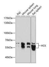
Western blot analysis of various lysates using HCK Rabbit pAb (A14537) at 1:1000 dilution. Secondary antibody: HRP-conjugated Goat anti-Rabbit IgG (H+L) (AS014) at 1:10000 dilution. Lysates/proteins: 25µg per lane. Blocking buffer: 3% nonfat dry milk in TBST. Detection: ECL Basic Kit (RM00020). Exposure time: 90s.
